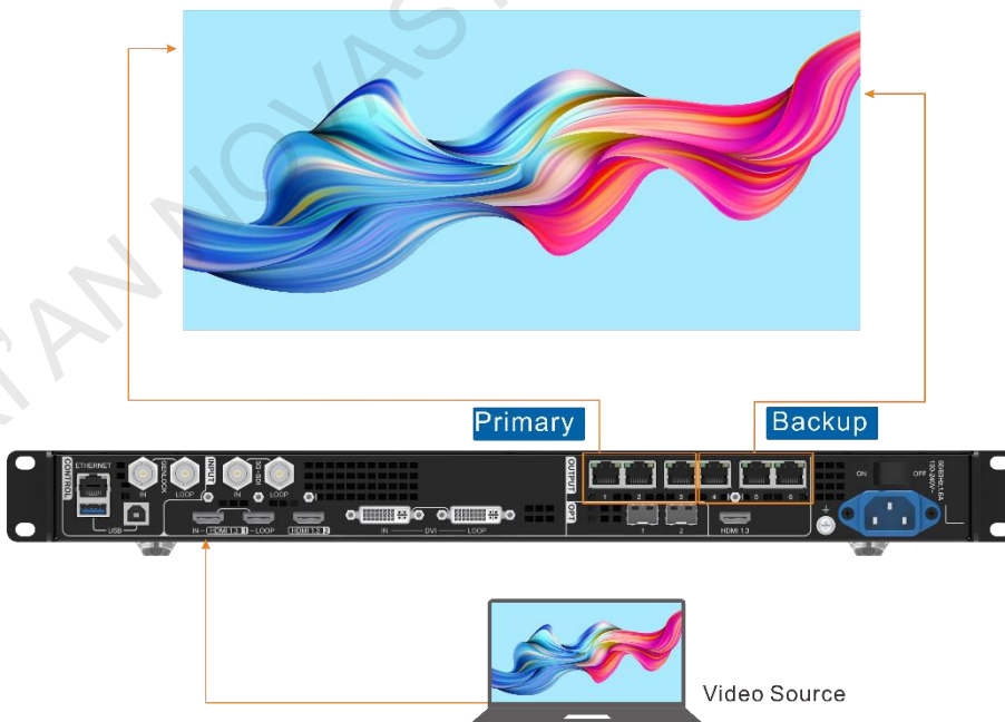
Figure 5-27 Ethernet port backup connection
