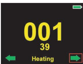
The fixture is waiting for reaching operating temperature of the fixture inside (inside temperature is below 0°C). Fixture does not respond to DMX.
