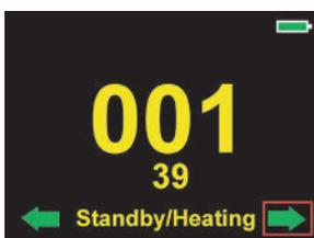
The fixture is in standby mode and inside of the fixture is heated (ambient temperature is below 0°C). Fixture does not respond to DMX, but display is active. Fixture sends its statuses and recorded physical values ( temperature, humidity, pressure) to the REAP.
