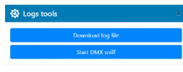
"Download log file" - the option allows you to download the log file to computer, name of the log file is: file-abcd.log, where abcd is a fixture ID (e.g. file-015e.log).
