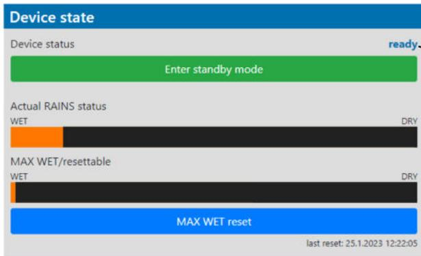
Device status **ready** means, that all fixture resets are OK and the fixture is ready for operation. It does not assess state of desiccants or result of pressure test!
