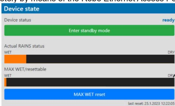
The chart MAX WET is decisive for replacing desiccant in the fixture arm. If the chart has changed to black colour, desiccant has to be replaced.
