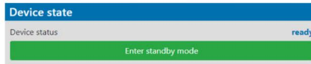
Note: Standby mode helps conserve power when a fixture is not in use, without fully powering it off. In the Standby mode, all fixture motors and fans are deactivated and light output is closed. For more information about Standby mode please see the chapter Standby mode.
