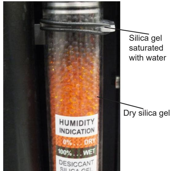
To change the tube with the silica gel in the fixture arm.
