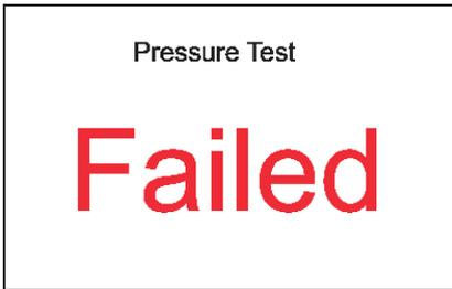
If the first pressure test failed and the second is OK, the fixture complies with IP65 integrity. If the pressure test twice fails despite checking of correct tightening of the cover screws and gaskets under covers, the fixture has to be tested by means of "Enhanced pressure test". For this type of pressure test is needed the Pressure IP Testing Set ROBE (P/N 10980659). Please ask your ROBE distributor for help.
